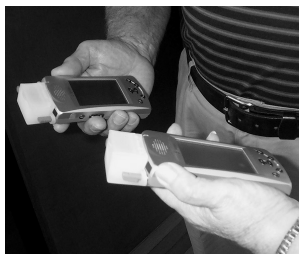
Fig. 1. The PDA Pillbox Prototype (patent pending) on the Samsung i300. The pillbox could hold a day's worth of pills, improved stylus access, and allowed wireless infrared transfer.
